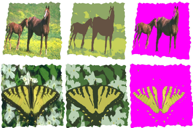
Figure 6: Segmentation results on meshes in the multi-region case. Top row: Horse data set and its segmentation for three regions. Bottom row: Four regions labeling of the Butterfly data. (a) Input textured mesh; (b) Recovered mean values of each region obtained by our approach; (c) One of the segmented regions.
