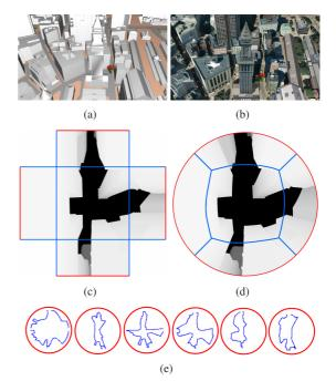
Figure 5. Our algorithm to construct a fisheye image. (a) and (b) show the 3D model and aerial image of an urban scene where we synthesize a fisheye image. (c) The cubemap generated from a given point in the 3D model. Note that in practice, we generate binary images; the slight shading here is just for visualization. (d) Fisheye image created from the cubemap. (e) Examples of skylines extracted from the fisheye images.
