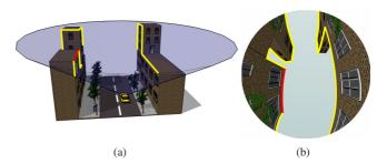
Figure 1. An illustration of our motivating idea. (a) A car automounted with an omni-directional camera facing towards the sky. (b) The image captured by the camera with skylines marked. We match these skylines to those synthesized from 3D city models to compute the geospatial location.
