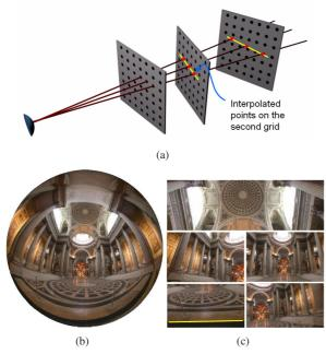
Figure 4. (a) Generic calibration using three calibration grids. (b) and (c) show an original fisheye image and samples of distortion corrected regions, obtained using the calibration result.
