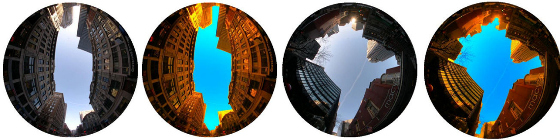
Figure 7. Sky detection results: Original and segmented fisheye images are shown.
