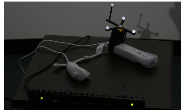
Figure 18: Optically tracked Nintendo wiimote
