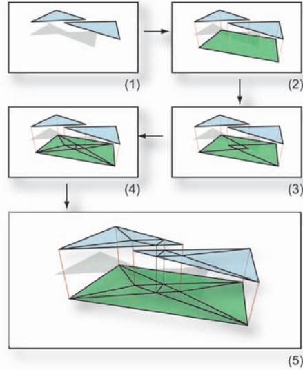
Figure 1: Different steps of the 3D subdivision process.
