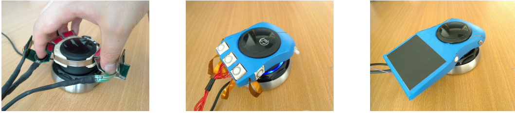
Figure 1: From left to right: the V2 prototype with petals and force sensors, the V3c prototype with trackballs and the V3b prototype with a touchpad and trackballs.
