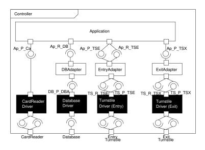
Fig. 3. Software architecture of the access control system.
