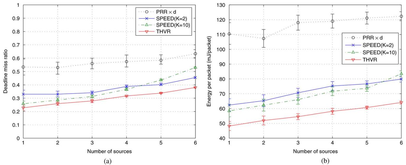
Fig. 7. Performance of: (i) (PRR  $\times$  d)-routing; (ii) SPEED; and (iii) THVR, each with 90% confidence interval indicated, while the number of source nodes increases from 1 to 6. (a) DMR with number of sources varied. (b) Energy consumed per successfully transmitted packet.
