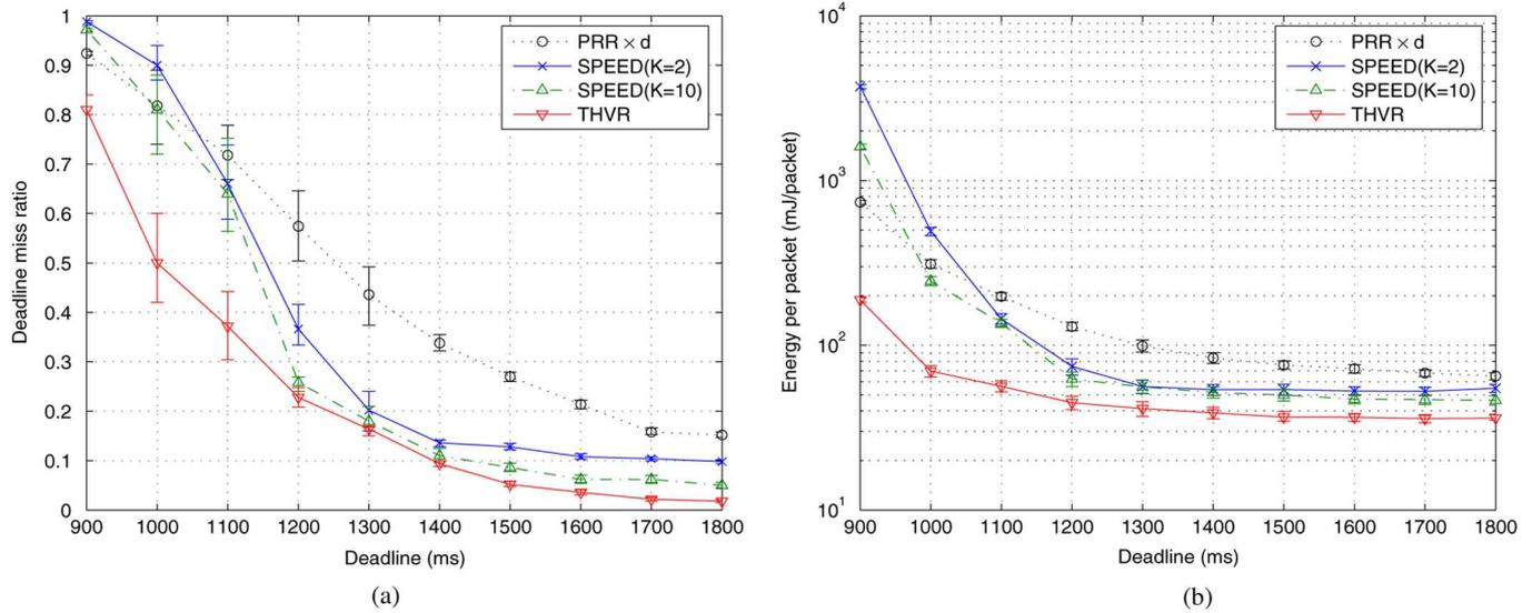
Fig. 6. Performance of: (i) PRR-distance-product routing; (ii) SPEED, with  $K = 2$  and 10 in (5), respectively; and (iii) THVR, each with 90% confidence interval. (a) DMR with deadline varied. (b) Energy consumed per successfully transmitted packet.
