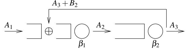
**Figure 6. Feedback control to ensure non-overflow for the second buffer.**
