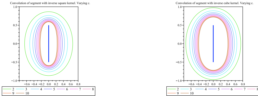
Fig. 3. Different level sets for the convolution function obtained for a fixed line segment with a square (left) and cubic (right) power inverse kernel.
