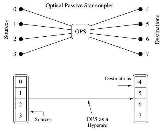
Figure 3: Modeling an OPS by a hyperarc.
