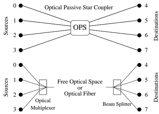
Figure 2: A degree 4 optical passive star coupler.
