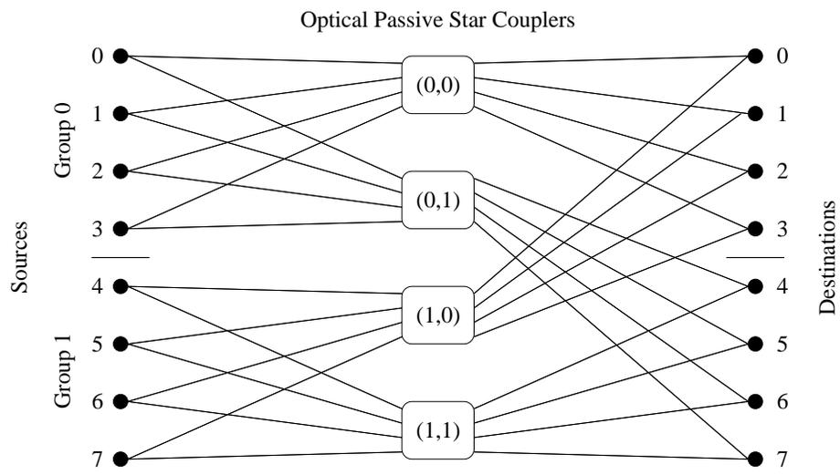
Figure 4: Partitioned Optical Passive Star POPS(4,2) with 8 nodes.
