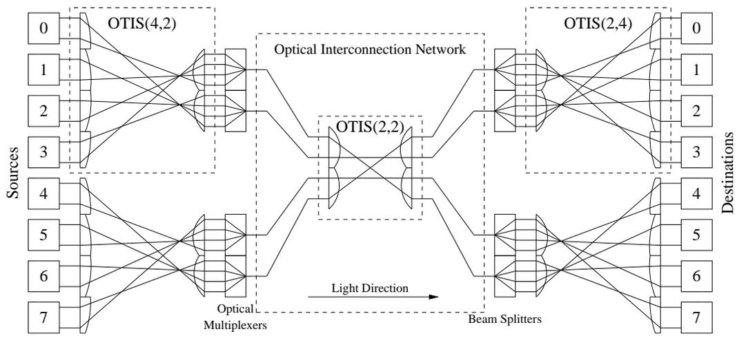
Figure 13: Optical interconnections of  $POPS(4,2)$  using the OTIS architecture.
