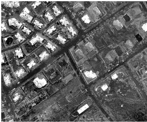
(c) The a^* channel in the CIE L^*a^*b^* color space
