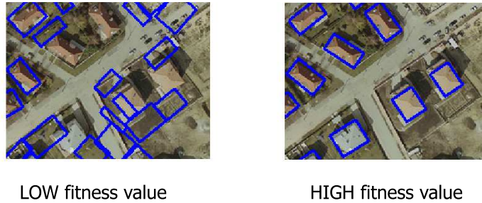
Figure 2: Demonstration of inverse techniques. The fitness function can be evaluated for each possible object configuration, however, it must result in a low fitness value for incorrect populations (left), and a high fitness value for the relevant ones (right)
