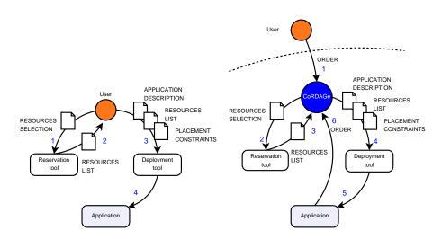
FIG. 1 – Deploying an application (a) by hand, and (b) using the CORDAGE tool.
