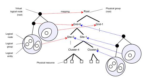
FIG. 2 - Two ways of mapping the same logical tree on the physical resource tree. Left is top-most, which ensures a greater distribution of entities over resources. Right is bottom-most, used to deploy entities on resources as close as possible.
