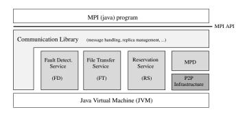
Figure 2. P2P-MPI structure.
