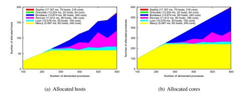
Figure 4. Hosts and cores allocated with Concentrate
