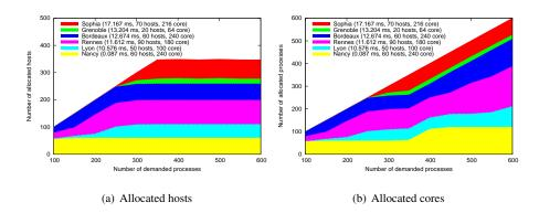
Figure 5. Hosts and cores allocated with Spread
