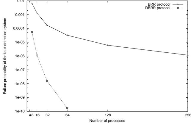
**Figure 12.** Failure probabilities of the FD system using BRR and DBRR ( $\delta = 1$ ,  $\lambda t = 10^{-1}$ ).
