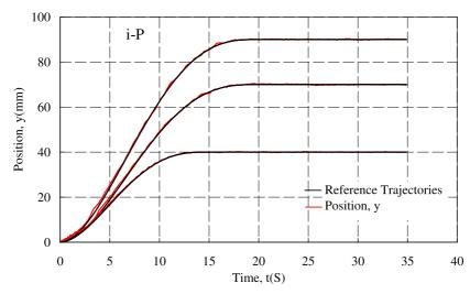
Fig. 4. Classical tracking when the actuator is controlled with an *i*-P controller.
