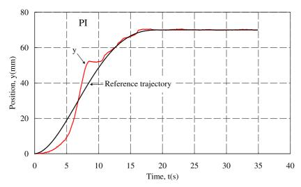
Fig. 5. Classical tracking when the actuator is controlled with a PI controller.
