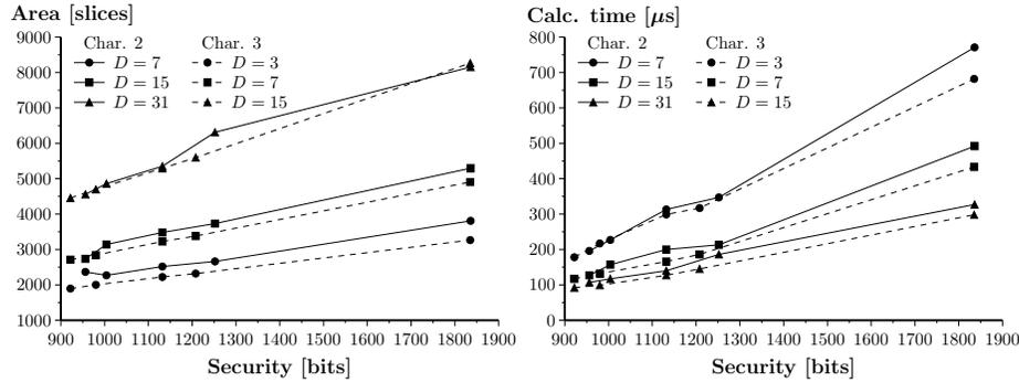
**Fig. 1.** Area (left) and calculation time (right) for the modified Tate pairing on our unified operator, in both characteristics two and three, for various extension degrees and different values for the parameter  $D$ .
