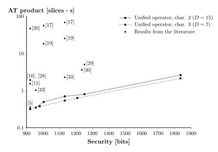
Fig. 2. Area-time product of the proposed coprocessor for the modified Tate pairing in characteristics two and three against the other solutions published in the literature.
