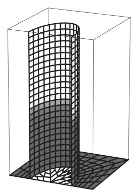
Figure 4. Fibre-reinforced material: representative cell, damaged zones.
