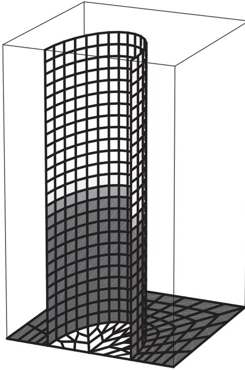
Figure 4. Fibre-reinforced material: representative cell, damaged zones.
