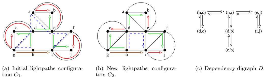
Figure 1: Example of an instance of the reconfiguration problem consisting of a network with 10 nodes and symmetric arcs, 8 connections  $(h, i)$ ,  $(h, c)$ ,  $(d, c)$ ,  $(d, b)$ ,  $(e, b)$ ,  $(e, j)$ ,  $(i, j)$ ,  $(g, i)$  to be established. Fig. 1(a) depicts the initial configuration  $C_1$ , Fig. 1(b) the new configuration  $C_2$ , and Fig. 1(c) the dependency digraph from  $C_1$  to  $C_2$ .
