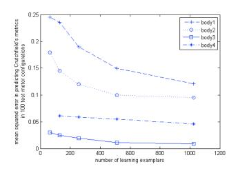
Fig. 8. Evolution of mean squared errors in predicting Crutchfield's metrics between the two sensors of bodies 1, 2, 3 and 4 when various number of learning examplars are available (each learning examplar is an association between a random motor configuration and the associated measured Crutchfield informational distance) and with a test database composed of 100 motor configurations uniformly spread in the space of configurations.
