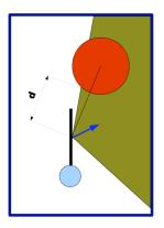
Fig. 3. **Distance sensor.** The location and orientation of the sensor are represented by the blue arrow. The perceived distance  $\mathbf{d}$  correspond to the distance between the origin of the sensor and the nearest object of the environment within the perceptive field of the sensor (yellow-green area).
