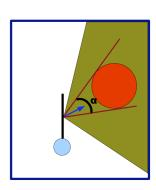
Fig. 4. **Apparent angle sensor.** The location and orientation of the sensor are represented by the blue arrow. Perceive the angle  $\alpha$  under which is seen from the sensor the closest object of the environment within its perceptive field.
