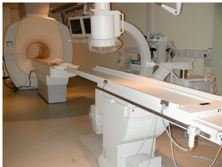
Fig 2a: Hybrid x-ray / MR system
