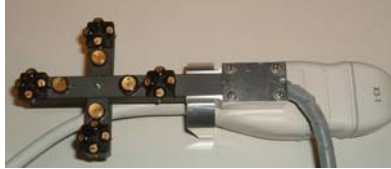
Fig. 5. Tracking the 3D echo probe by using Optotrak system.
