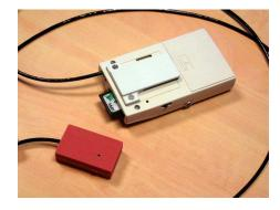
Fig. 1. The CEA-LETI Attitude Sensor with its Data Processing Unit
