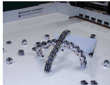
Fig. 1. A model of aggregated swarm robots in the SYMBRION project.
