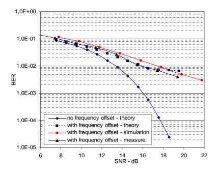
Figure 5 – Frequency offset impact on AWGN SISO BER performances (theoretical, simulated and measured data). The frequency offset value is  $20 \, \mathrm{kHz}$ .
