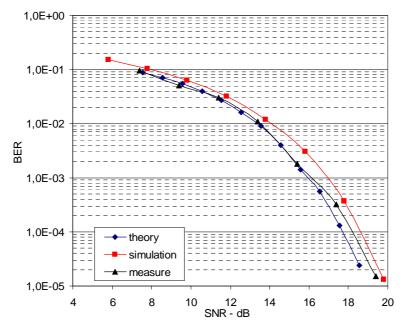
Figure 2 - Uncoded 802.11g AWGN BER performances. Theoretical, simulated and measured data are plotted versus SNR.
