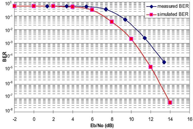
Fig. 5. BER vs.  $E_b/N_0$  in AWGN channel
