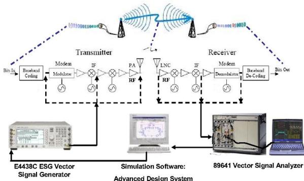
Fig. 1. The platform structure for a 1x1 transmission
