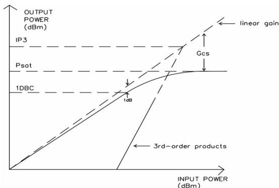
Fig. 8 Nonlinear element characterization for nonlinear models
