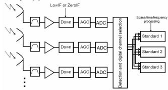
Figure 1: General architecture of a multi-\* SDR receiver
