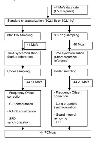
Figure 2: General structure of the software WLAN receiver
