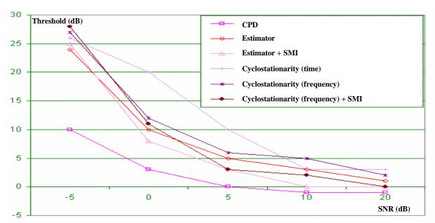
Figure 4: Obtained detection threshold in a multipath channel versus signal to noise ratio with different methods
