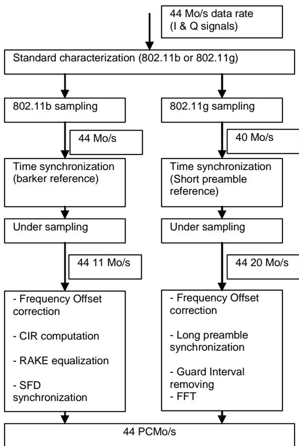
Figure 2: General structure of the software WLAN receiver
