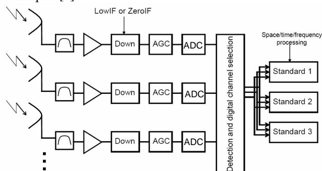
Figure 1: General architecture of a multi-\* SDR receiver
