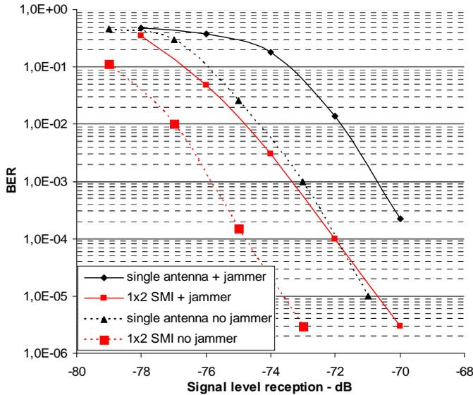
Figure 7: 802.11g suffering from 802.11b interference performances
