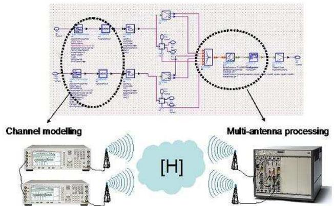
Figure 1: 2x2 MIMO transmission with the radio platform
