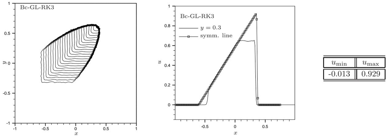
Figure 24: 2d Burger's equation : Bc-GL-RK3 scheme. Left : contours at time  $t = 1$ . Middle : solution along the line  $y = 0.3$  and along the symmetry line. Right : minimum and maximum values of the solution.
