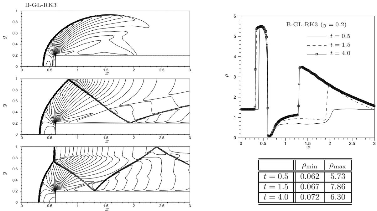
Figure 37: Mach 3 wind tunnel : B-GL-RK3 scheme. Left : density contours at time  $t = 0.5$  (top),  $t = 1.5$  (middle), and  $t = 4.0$  (bottom) ; 30 equally spaced contours between 0.5 and 8. Right : density distribution along the line  $y = 0.2$ , and minimum and maximum values of the density.
