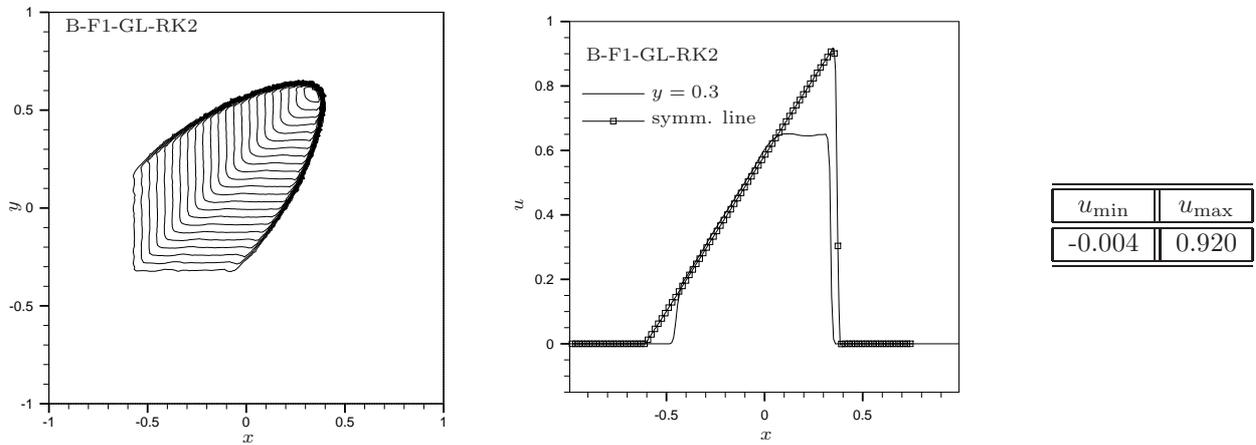
Figure 14: 2d Burger's equation : B-F1-GL-RK2 scheme. Left : contours at time  $t = 1$ . Middle : solution along the line  $y = 0.3$  and along the symmetry line. Right : minimum and maximum values of the solution.
