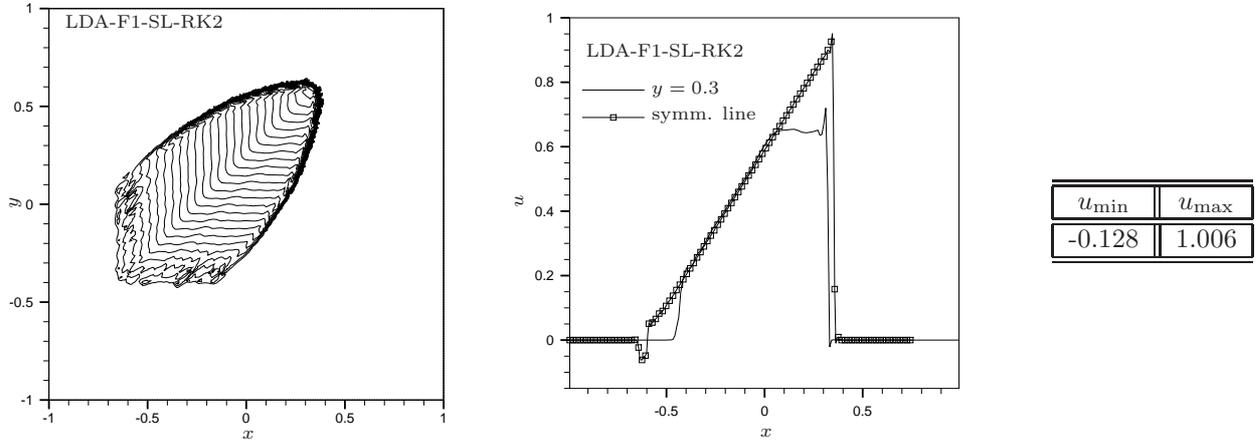
Figure 9: 2d Burger's equation : LDA-F1-SL-RK2 scheme. Left : contours at time  $t = 1$ . Middle : solution along the line  $y = 0.3$  and along the symmetry line. Right : minimum and maximum values of the solution.
