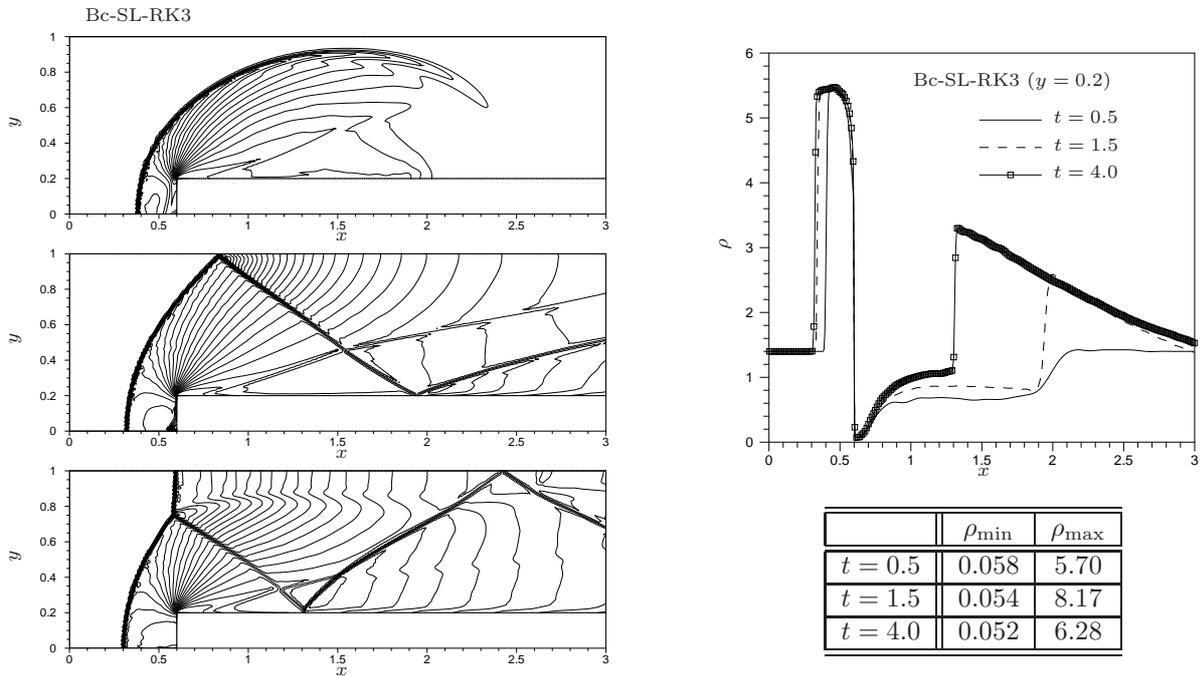
Figure 39: Mach 3 wind tunnel : Bc-SL-RK3 scheme. Left : density contours at time  $t = 0.5$  (top),  $t = 1.5$  (middle), and  $t = 4.0$  (bottom) ; 30 equally spaced contours between 0.5 and 8. Right : density distribution along the line  $y = 0.2$ , and minimum and maximum values of the density.
