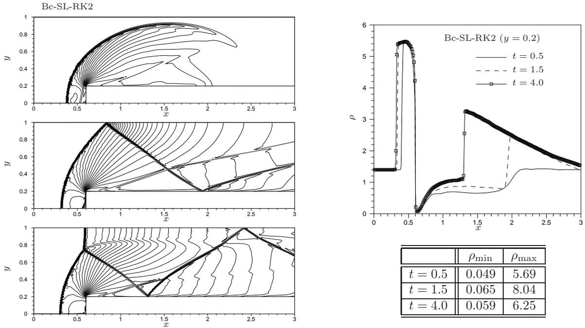
Figure 38: Mach 3 wind tunnel : Bc-SL-RK2 scheme. Left : density contours at time  $t = 0.5$  (top),  $t = 1.5$  (middle), and  $t = 4.0$  (bottom) ; 30 equally spaced contours between 0.5 and 8. Right : density distribution along the line  $y = 0.2$ , and minimum and maximum values of the density.
