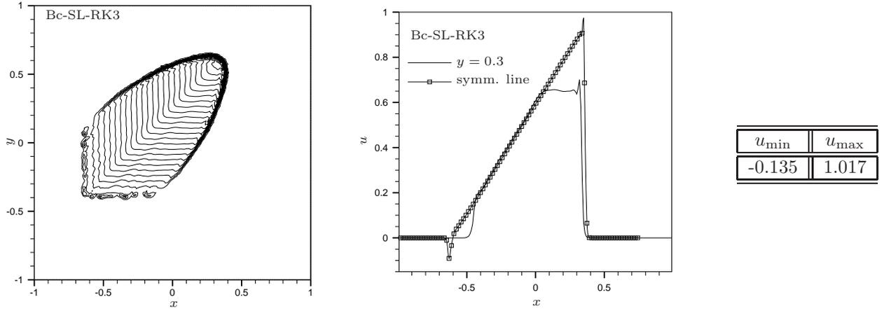
Figure 23: 2d Burger's equation : Bc-SL-RK3 scheme. Left : contours at time  $t = 1$ . Middle : solution along the line  $y = 0.3$  and along the symmetry line. Right : minimum and maximum values of the solution.
