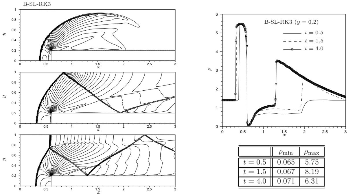
Figure 35: Mach 3 wind tunnel : B-SL-RK3 scheme. Left : density contours at time  $t = 0.5$  (top),  $t = 1.5$  (middle), and  $t = 4.0$  (bottom) ; 30 equally spaced contours between 0.5 and 8. Right : density distribution along the line  $y = 0.2$ , and minimum and maximum values of the density.
