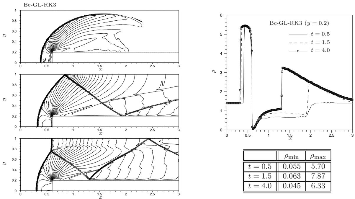
Figure 41: Mach 3 wind tunnel : Bc-GL-RK3 scheme. Left : density contours at time  $t = 0.5$  (top),  $t = 1.5$  (middle), and  $t = 4.0$  (bottom) ; 30 equally spaced contours between 0.5 and 8. Right : density distribution along the line  $y = 0.2$ , and minimum and maximum values of the density.
