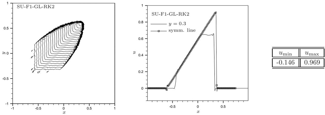
Figure 18: 2d Burger's equation : SU-F1-GL-RK2 scheme. Left : contours at time  $t = 1$ . Middle : solution along the line  $y = 0.3$  and along the symmetry line. Right : minimum and maximum values of the solution.
