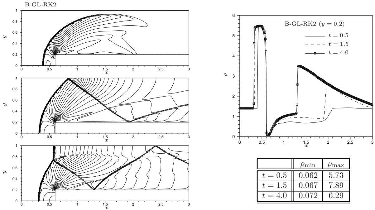
Figure 36: Mach 3 wind tunnel : B-GL-RK2 scheme. Left : density contours at time  $t = 0.5$  (top),  $t = 1.5$  (middle), and  $t = 4.0$  (bottom) ; 30 equally spaced contours between 0.5 and 8. Right : density distribution along the line  $y = 0.2$ , and minimum and maximum values of the density.
