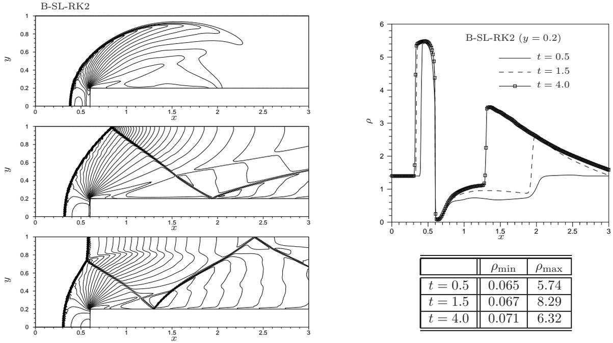
Figure 34: Mach 3 wind tunnel : B-SL-RK2 scheme. Left : density contours at time  $t = 0.5$  (top),  $t = 1.5$  (middle), and  $t = 4.0$  (bottom) ; 30 equally spaced contours between 0.5 and 8. Right : density distribution along the line  $y = 0.2$ , and minimum and maximum values of the density.
