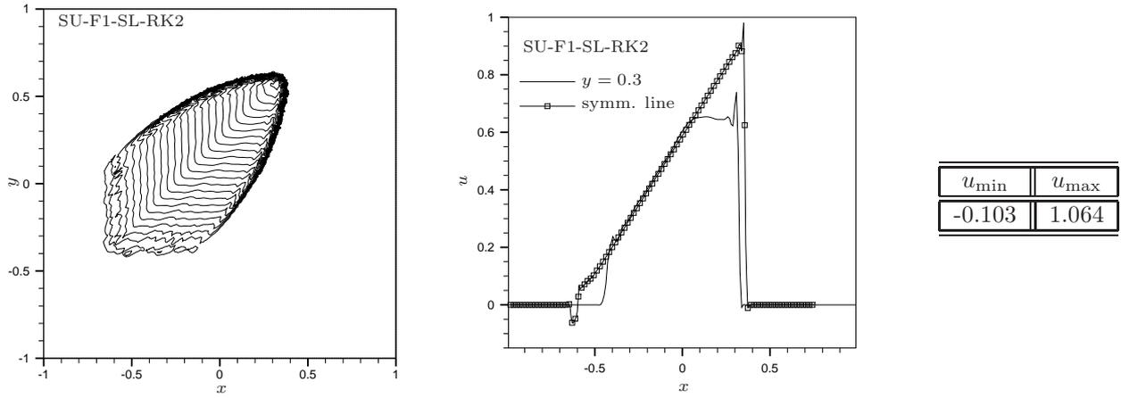
Figure 17: 2d Burger's equation : SU-F1-SL-RK2 scheme. Left : contours at time  $t = 1$ . Middle : solution along the line  $y = 0.3$  and along the symmetry line. Right : minimum and maximum values of the solution.
