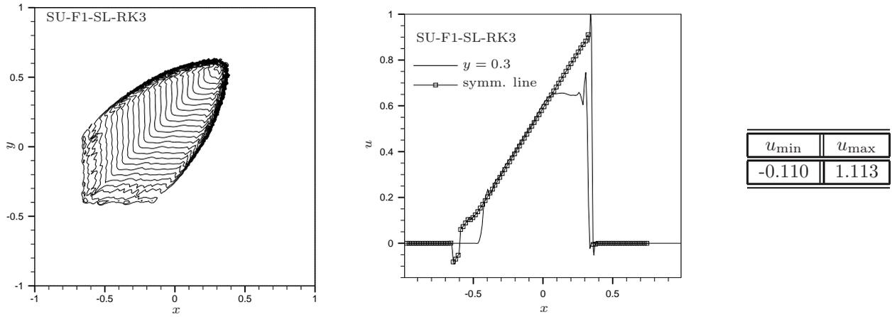
Figure 19: 2d Burger's equation : SU-F1-SL-RK3 scheme. Left : contours at time  $t = 1$ . Middle : solution along the line  $y = 0.3$  and along the symmetry line. Right : minimum and maximum values of the solution.
