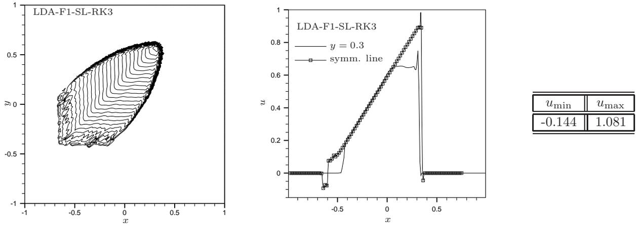
Figure 11: 2d Burger's equation : LDA-F1-SL-RK3 scheme. Left : contours at time  $t = 1$ . Middle : solution along the line  $y = 0.3$  and along the symmetry line. Right : minimum and maximum values of the solution.
