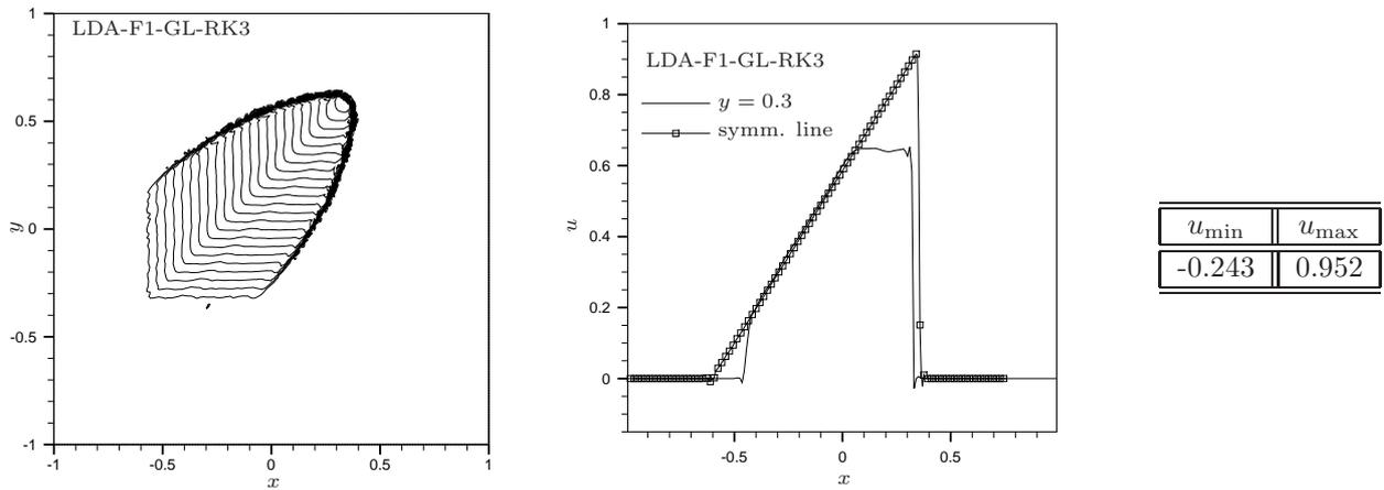
Figure 12: 2d Burger's equation : LDA-F1-GL-RK3 scheme. Left : contours at time  $t = 1$ . Middle : solution along the line  $y = 0.3$  and along the symmetry line. Right : minimum and maximum values of the solution.
