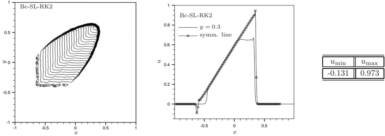
Figure 21: 2d Burger's equation : Bc-SL-RK2 scheme. Left : contours at time  $t = 1$ . Middle : solution along the line  $y = 0.3$  and along the symmetry line. Right : minimum and maximum values of the solution.
