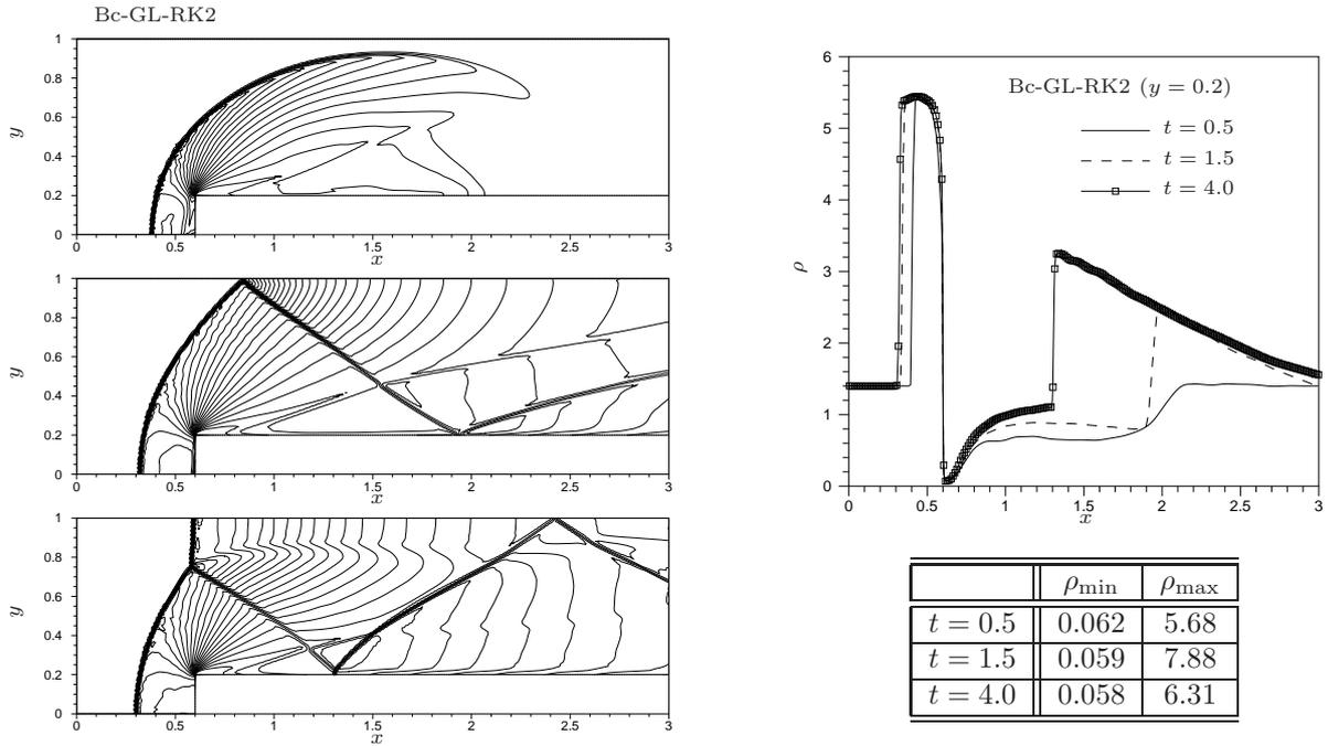
Figure 40: Mach 3 wind tunnel : Bc-GL-RK2 scheme. Left : density contours at time  $t = 0.5$  (top),  $t = 1.5$  (middle), and  $t = 4.0$  (bottom) ; 30 equally spaced contours between 0.5 and 8. Right : density distribution along the line  $y = 0.2$ , and minimum and maximum values of the density.
