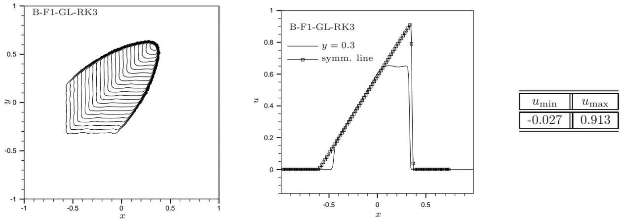
Figure 16: 2d Burger's equation : B-F1-GL-RK3 scheme. Left : contours at time  $t = 1$ . Middle : solution along the line  $y = 0.3$  and along the symmetry line. Right : minimum and maximum values of the solution.
