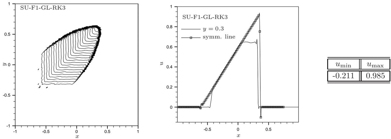
Figure 20: 2d Burger's equation : SU-F1-GL-RK3 scheme. Left : contours at time  $t = 1$ . Middle : solution along the line  $y = 0.3$  and along the symmetry line. Right : minimum and maximum values of the solution.
