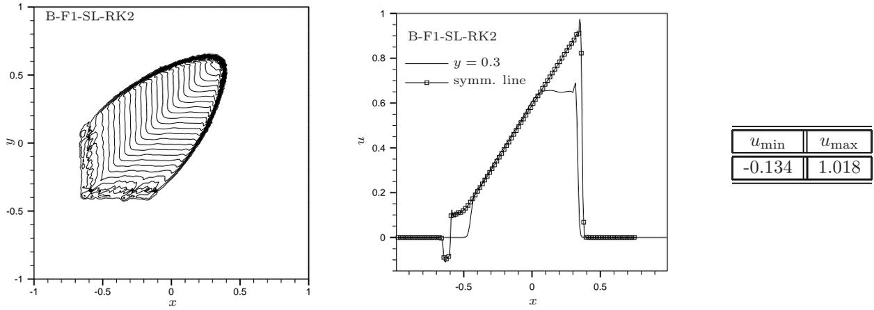
Figure 13: 2d Burger's equation : B-F1-SL-RK2 scheme. Left : contours at time  $t = 1$ . Middle : solution along the line  $y = 0.3$  and along the symmetry line. Right : minimum and maximum values of the solution.
