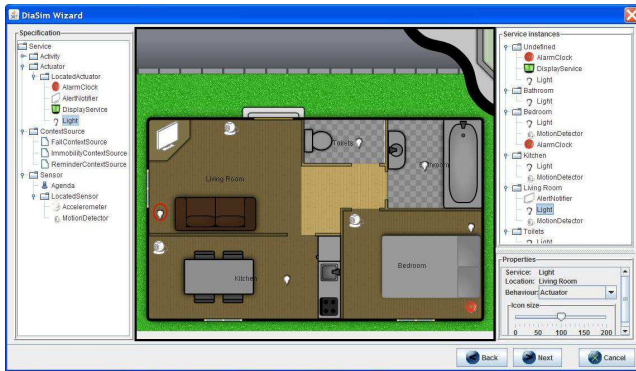
Figure 13. DiaSim simulated environment editor for an health care scenario. The middle frame displays a 2D view of a home environment. The devices extracted from a DiaSpec taxonomy are displayed on the left frame and can be placed via drag-and-drop operations in the simulated environment. The right frame summarizes devices deployed in the environment.
