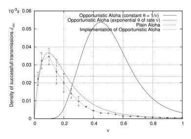
Fig. 16.2 The density of successful transmissions  $d_{suc}$  of Opportunistic Aloha for various choices of  $\theta$ . The propagation model is (16.1). We assume Rayleigh fading with mean 1 and  $W=0, \lambda=0.001, T=10 {\rm dB}, r=\sqrt{1/\lambda}$  and  $\beta=4$ . For comparison the constant value  $\lambda_{\rm max} p_c(r,\lambda_{\rm max})$  of plain Aloha is plotted.
