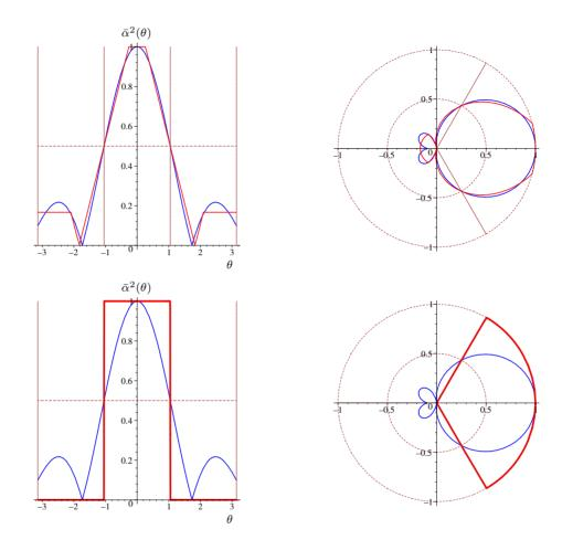
Fig. 22.1 Top: approximation of RP1 by RP2 with  $\theta_1=\frac{1}{12}\pi,\theta_2=\frac{2}{3}\pi;$  Cartesian and polar plots. Bottom: in boldface/red, perfect RP modeled by RP2 with  $\theta_1\to\pi/3-$  and  $\theta_2\to\pi/3+;$  Cartesian and polar plots.
