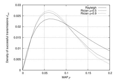
Fig. 16.3 Density of successful transmissions  $d_{suc}$  for plain Aloha in function of p in the Rayleigh and the Rician (with q=1/2 and q=.9) fading cases;  $\lambda=r=1, W=0$ , and T=10dB,  $\beta=4$ .
