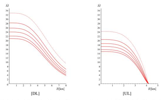
Fig. 18.2 Maximal load estimations in Honeycomb model at a given CPR  $\epsilon = 0.2, 0.1, 0.05, 0.02, 0.01$  (solid lines) for the downlink (DL) and uplink (UL). The dashed curves represent the values for the mean model. The numerical assumptions are as on Figure 18.1. User maximal power constraints are taken into account on UL as proposed in (Baccelli, Błaszczyszyn, and Karray 2004).
