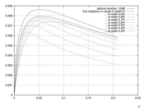
Fig. 16.7 Density of directional progress for the  $\frac{M}{0+M/M}$  model with OPL 3 with  $\beta=3, \lambda=1$ , with T=10dB. Comparison of the opportunistic and the "smallest hop in a cone" cases.
