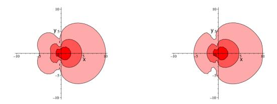
Fig. 22.2 Equal-strength power sets (path-loss level sets) for (c) with omnidirectional attenuation OPL 2 with  $A=1000, \beta=3$ , and radiation patterns RP1 (left), RP2;  $\theta_1=\frac{1}{12}\pi, \theta_2=\frac{2}{3}\pi$  (right). The contours represent the levels  $t=\{100,110,120\}$ dB.
