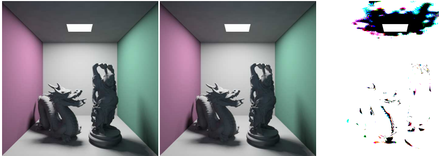
Figure 2: Geometric robustness when using direct access. (Left) The precomputation is performed in 58s on a low detailed geometry (24K triangles) and (Center) and in 180s high detailed geometry (2M triangles). (Right) The difference color-coded RGB image (maximum pixel difference is \varepsilon = 1.5\% ).
