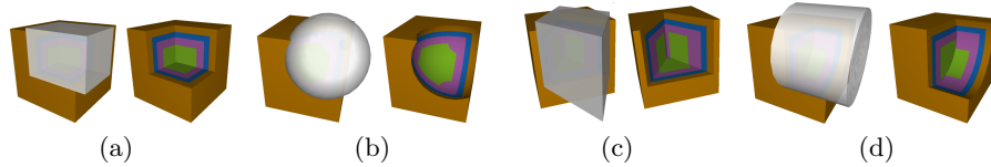
Fig. 3. Cut shapes and their resulting cutaway, (a) cubic cut shape, (b) spherical cut shape, (c) wedge cut shape, (d) tube cut shape.
