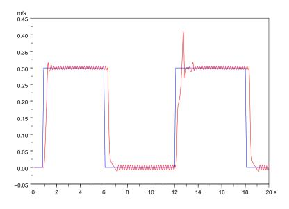
Figure 2: Forward speed of the CoM (red) and reference speed (blue) for the motion of Fig. 1.
