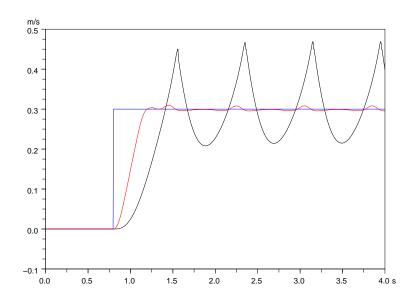
Figure 7: Comparison between the forward speed obtained with our method (red) and with the method proposed in [11] (black) when the reference speed (blue) is changed from 0 to  $0.3 \text{ ms}^{-1}$  at the beginning of a step.
