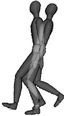
Fig. 2. 22 degrees of rotation of the whole body in the sagittal plane induced by 24 steps of the walking pattern recorded in [31] and replayed on a simple free-floating biomechanical model, what corresponds to a complete turn in 393 steps.
