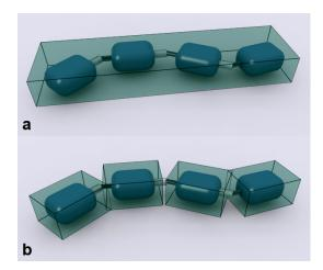
Figure 5: Visibility estimation from bounding volumes The visibility estimation  $N_{\mathbf{M}}(C)$  is taken as the minimum of two projections. a: Projected bounding volume of the entire articulated body. b: Sum of the projected bounding volumes of individual rigid bodies.
