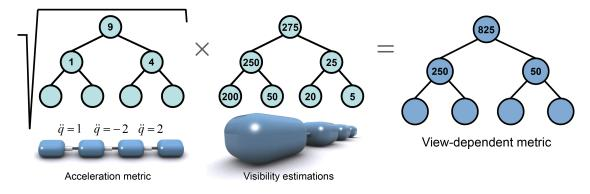
Figure 4: **View-dependent motion metric.** The view-dependent motion metric is obtained by combining a priori motion metrics with visibility estimations.
