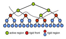
Figure 3: **Assembly tree of an articulated body.** Adaptive articulated-body dynamics simulates only some of the joints in the articulated bodies, which form the *active region*.
