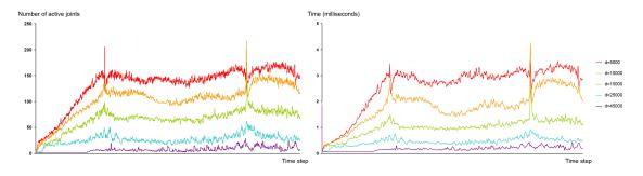
Figure 9: **Performance of our algorithm depending on the viewer's distance.** Our algorithm automatically decreases the number of active joints when the distance d between the viewer and the pendulum increases (**left**), reducing the computational cost of the simulation (**right**).
