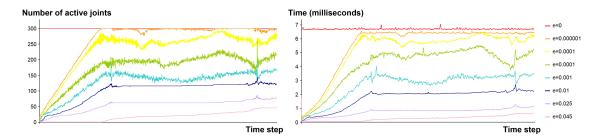
Figure 8: **Performance of our algorithm depending on visual error thresholds.** As the visual error threshold e increases, the number of active nodes is automatically decreased by the view-dependent algorithm (**left**), and the computational cost is reduced (**right**).
