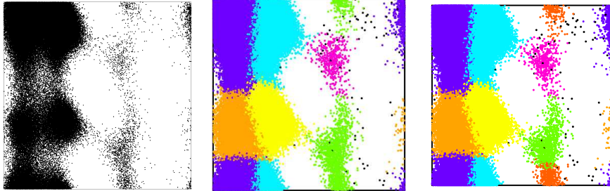
(a) Input point cloud after projection down to the (\phi, \psi) domain. (b) Segmentation with 6 clusters. (c) Segmentation with 7 clusters.
