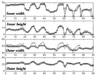
Figure 8. Results for the geometric features extraction. Reference measurements are plotted with crosses, tracking results are plotting with circle markers.
