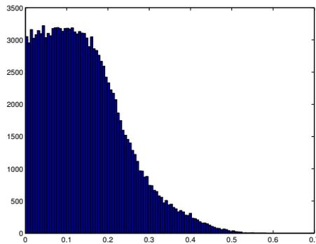
Fig. 4: **Point-plane distance.** Histogram of the distance in of each point to the linear least squares fitted plane (in millimeters) with the poses estimated with the three unknown mirror planes (section 4.1).
