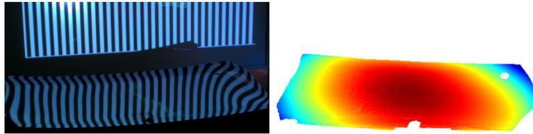
Fig. 5: **Real World Reconstruction.** Reconstruction of a car windshield. The method allowed us to easily obtain a 800 000 + point model using a classical video projector, on a large scale reflective surface. The hole in the middle is due to a non-specular patch on the surface.
