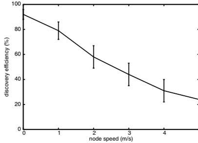
**Fig. 6.** Discovery efficiency in a mobile scenario
