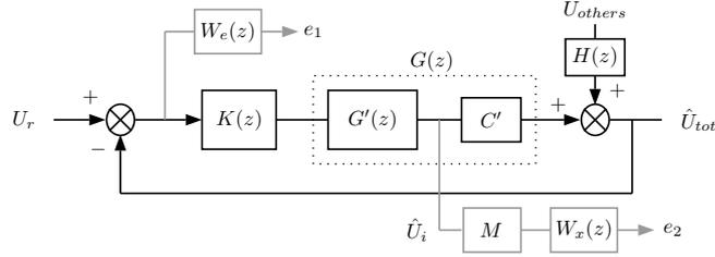
**Fig. 5.**  $H_\infty$  design bloc diagram
