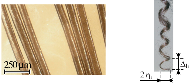
Figure 5: Left, measuring the mean radius r and the ellipticity e of the model by observation of real hair fibers with a video-microscope. Right, measuring the radius r_h and the step \Delta_h of the natural helical shape at the tip of a real hair clump.
