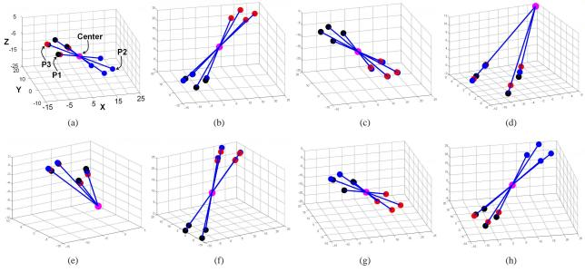
Figure 4. Calibration results for 3D central camera. Points of the same colour belong to a specific calibration grid. Eight possible solutions are shown. Two of the solutions shown in (d) and (e) satisfy the cheirality constraint.
