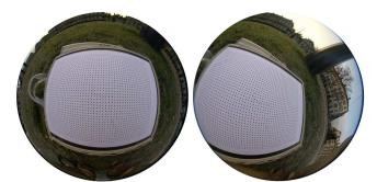
Figure 6. Two images of the grids used for calibrating the fisheye lens.
