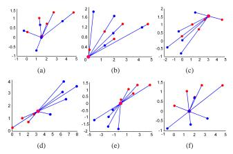
Figure 3. We show the calibration results. Points from a single calibration grid are represented by the same colour. Blue and Red color points refer to points on the first and the second calibration grids respectively. Six possible solutions are shown. The correct solution is the one shown in (b). In all other solutions the recovered points do not satisfy the cheirality constraint. (Best viewed in colour)
