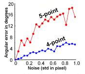
Figure 5. Comparison of 4-point and 5-point algorithms with respect to noise.
