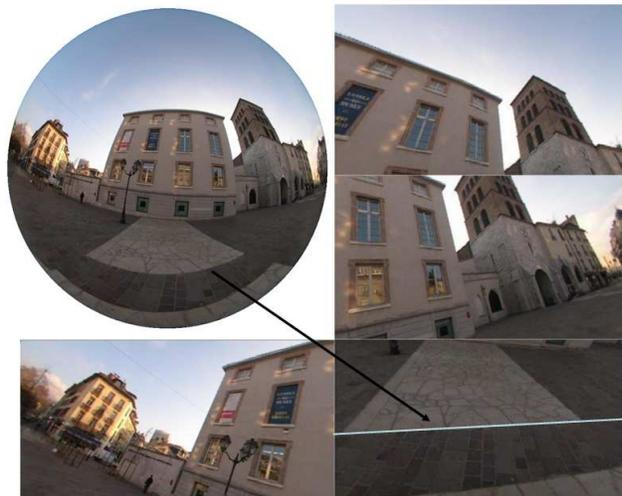
Figure 1. Distortion correction of a fisheye image after calibrating the camera using our 4-point algorithm. Note that the algorithm is capable of correcting highly distorted straight lines.
