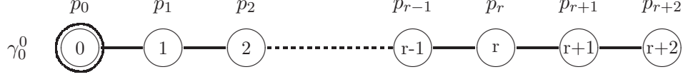
Figure 3: Initial configuration used in the proof of Proposition 4 (the numbers represent clock values and the double circles represent crashed processor).
