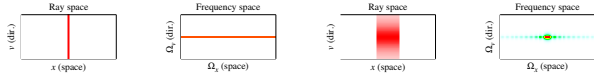
Figure 4: (a) A point light source is a Dirac in space times a constant in angle. (b) Its Fourier transform is a constant in space times a Dirac in angle. (c) A spot light with a finite-size bulb has a smooth falloff in angle. (d) Its Fourier transform is a sinc times a bell curve.
